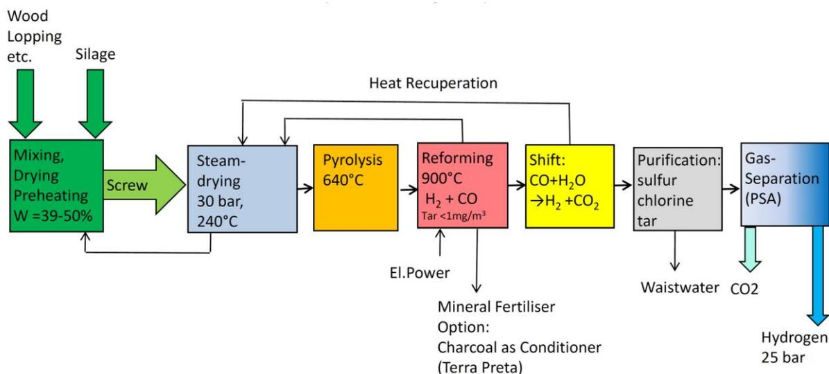
Fig. 8 Block Diagram of Hydrogen Production
